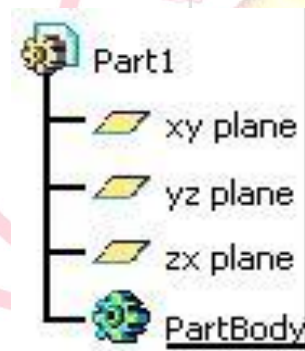
FIG.: The specification tree that appears on starting a new CAT Part file
